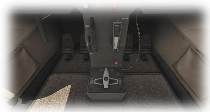
Center Console (Trim, and Fuel Selector)
